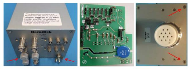
Figure 5.23: FT12TPz with internal HVZ board (#4) which is accessible after removing the bottom side of the case (loosen the four screws indicated by the red arrows). The rear detector potential is applied only via the U<sub>sig</sub> input.
