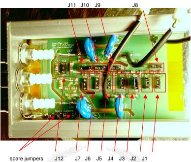
Figure 5.18: HVZ Revisions 1.3 and newer with jumper options.
