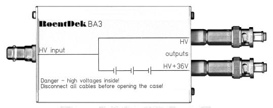
Figure 5.10: **RoentDek** BA3 battery box. The voltage input is on the left side, the output connectors (here as reserve SHV) on the right side. The input voltage is routed to the upper voltage output (for  $U_{ref}$ )) and produces with the internal battery pack the signal voltage  $U_{sig} = U_{ref} + 36 V$  (nominally) on the lower output connector. Newer versions of the BA3 have SHV sockets as outputs (instead of plugs shown here) and in-line 10 k $\Omega$  resistors.
