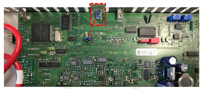
Figure 5.5: Photos of the internal circuit board (after opening the side panel). In big picture: standard jumper position for not enabling the "kill both" function (blue jumper not set, only "parked on one of the pins). Insert picture: Jumpers is set, bridging the pins for enabling "kill both" function.
