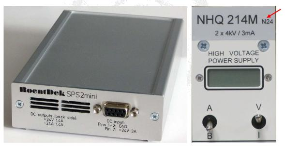
Figure 5.9: SPS2mini mains adapter (left) and the specific label (red arrow) on the front side of a "N24"- type HV2/4 module which can be powered by it (those units with side panel labels will show the N24 indication there). The N24-type HV modules can also be operated with old-type NIM-crates that does not supply the ±6 V.
