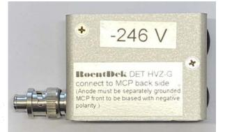
Figure 5.17 HVZ-G plug, here the version for negative bias of MCP back potential.
