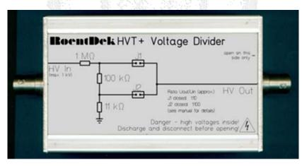
Figure 5.26: HVT+ with 100:10:1 resistor chain. Depending on the jumper the nominal scaling factor between output and input voltage is 1:10 (J1 set) or 1:100 (J2 set). The maximum input voltage is 1000 V. On demand the HVT+ can also come as a version equipped with a third jumper position J3 which enables the standard HVT functionality (see Chapter 5.5) with R<sub>HVT</sub> having a nominal value of 1111kΩ.
